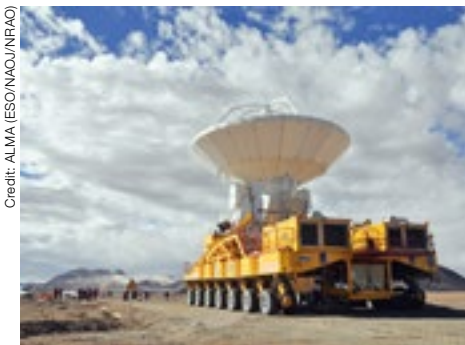
Figure 1. The transporter Otto is shown carrying one of the antennas from the OSF to the AOS. See Kraus et al. 2007 ( The Messenger , 132, 23) for more information on the ALMA transporters.
