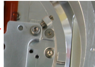
Mechanical Stop keeps X/Y alignment
